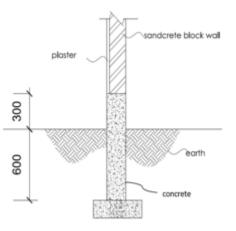
Fig 7. A schematic diagram of control test walls constructed without any treatment
