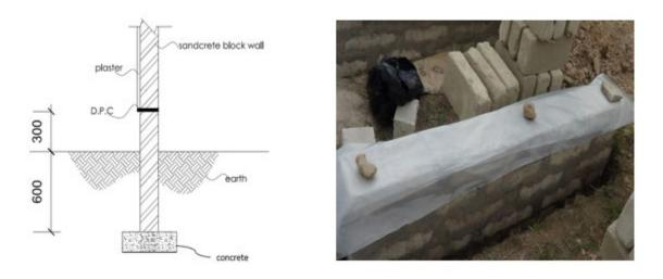
Fig 2 (a) Schematic diagram of the position of the dpc (b) Photograph showing how the dpc was laid (Source: Agyekum et al., 2016)
