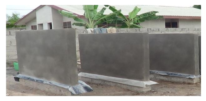
Fig 3 Photograph of test walls after the dpcs were laid
