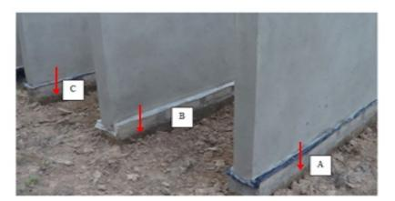
Fig 12 Water rise at the bases of the walls treated with three different DPCs - 0.15 mm thick (A), 0.12 mm thick (B) and 0.13 mm thick (C)
