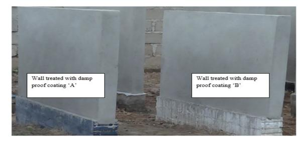
Fig 6 Photograph of test walls after they were treated with the damp proof coatings
