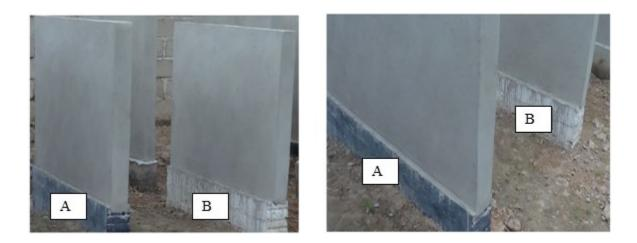
Fig 13a Photographs showing the conditions of the treated walls in the rainy season
