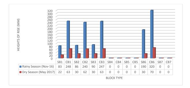
Fig 11c Capillary rise of water visually recorded at the peak of the seasons for 2016-2017
