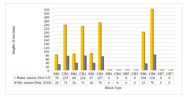
Fig 11b Capillary rise of water visually recorded at the peak of the seasons for 2015-2016
