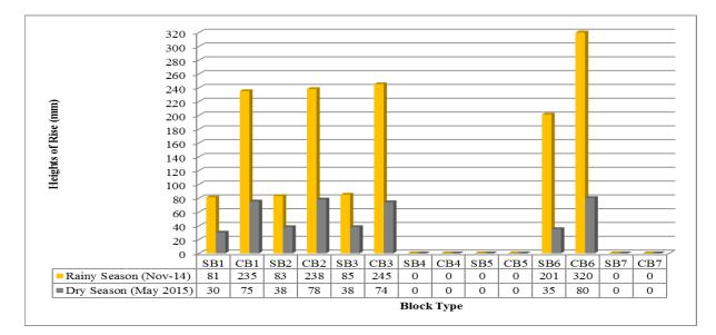
Fig 11a Capillary rise of water visually recorded at the peak of the seasons for 2014-2015
