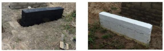
Fig 5 Photographs of the walls after the damp proof coatings 'A' (left) and 'B' (right) were applied
