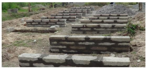
Fig 1 Photograph of test walls (extreme left are those constructed with SBs and extreme right are those constructed with CBs) (Source: Agyekum *et al.*, 2016)
