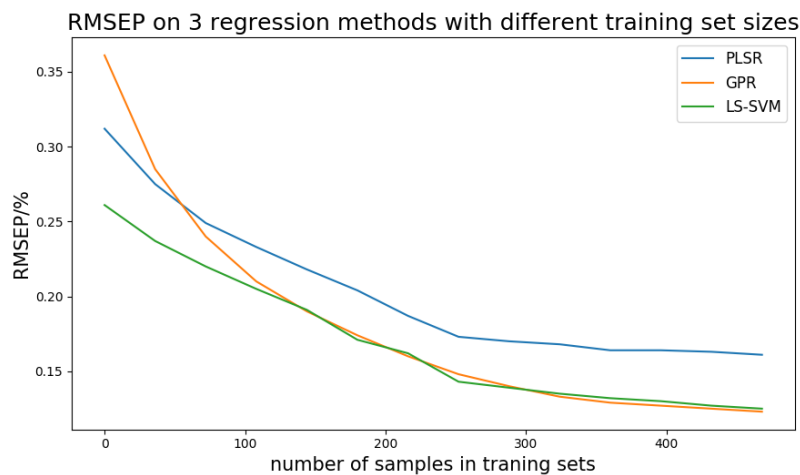
Figure 4.3: RMSEP for 3 models with varying training set size. PLSR: Cross-validations was performed to choose the number of factors for each test ; GPR and LS-SVM: RBF kernel.
