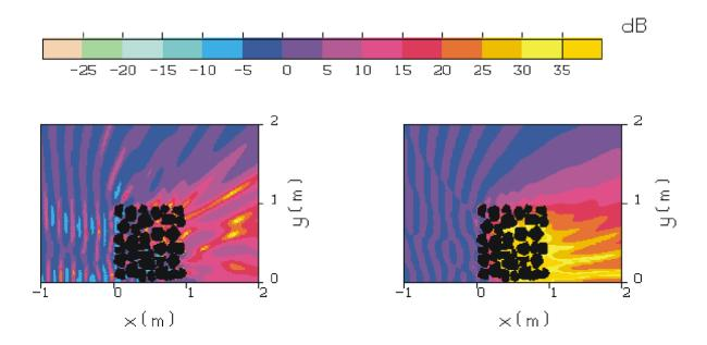
Figure 4. Insertion loss at 1000 Hz near a 1-m high and 1-m wide gabion barrier placed on rigid ground. On the left, rigid stones have been considered, on the right the equivalent case with expanded clay stones (flow resistivity of 82 kPas/m²) is depicted (From Ref. [49]).
