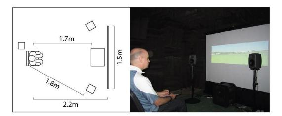
Figure 4. The layout of the anechoic chamber.
