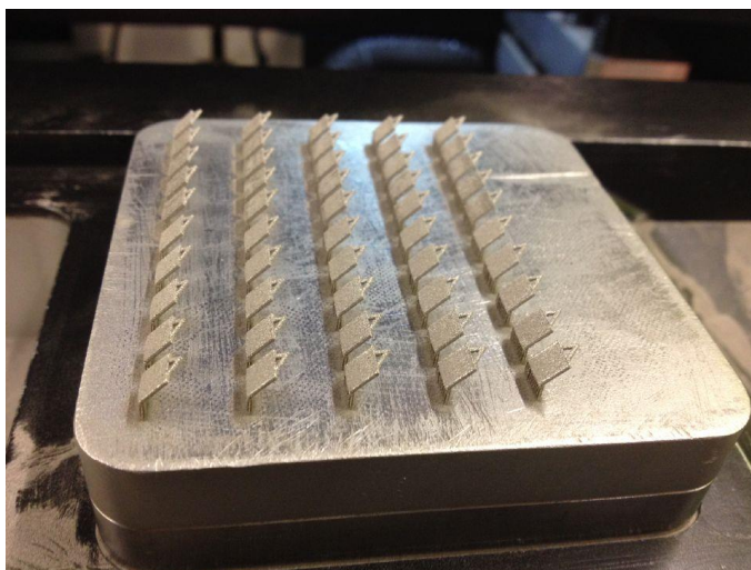
Figure S4. Photograph of 3D-printed stainless steel scaffolds fabricated using various laser power and scan rates.
