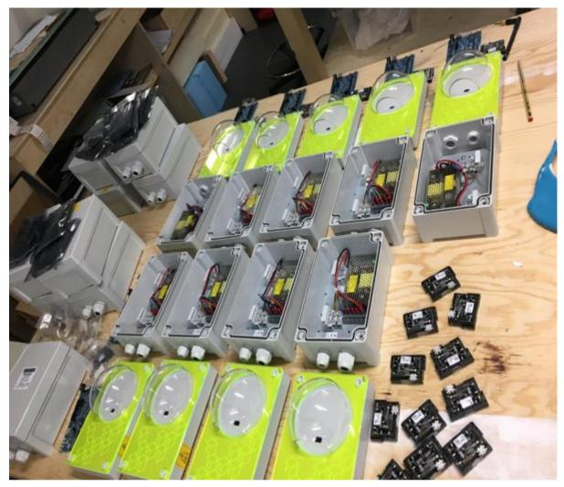
Figure 4 ICRI Environmental Sensor Assemblies.
