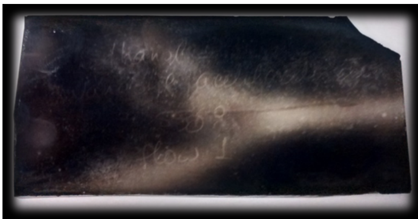
Figure 2.13: Black and non-uniform VO 2 film obtained by AACVD method (10X4cm)
