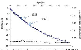
Fig. 5 Radiometric chronology of core MORAR2 taken from Loch Morar, Scotland, showing the CRS model <sup>210</sup>Pb dates, <sup>137</sup>Cs time markers, and sedimentation rates. The solid line shows age while the dashed line indicates sedimentation rate.
