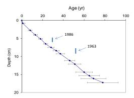
Fig 3 Radiometric chronology of core MORAR1 taken from Loch Morar, Scotland, showing the CRS model <sup>210</sup>Pb dates and the <sup>137</sup>Cs and <sup>241</sup>Am time markers
