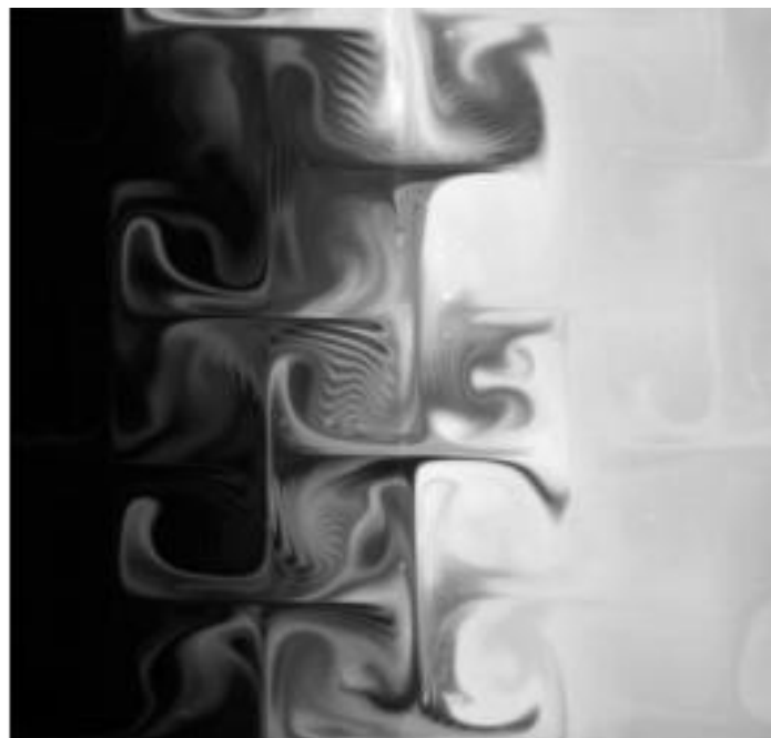
Figure 7.1 Snapshot of the concentration field for transient magnetically forced chaotic mixing. Fluid labelled with fluorescein was initially confined to the right half of the cell (Rothstein et al. 1999).
