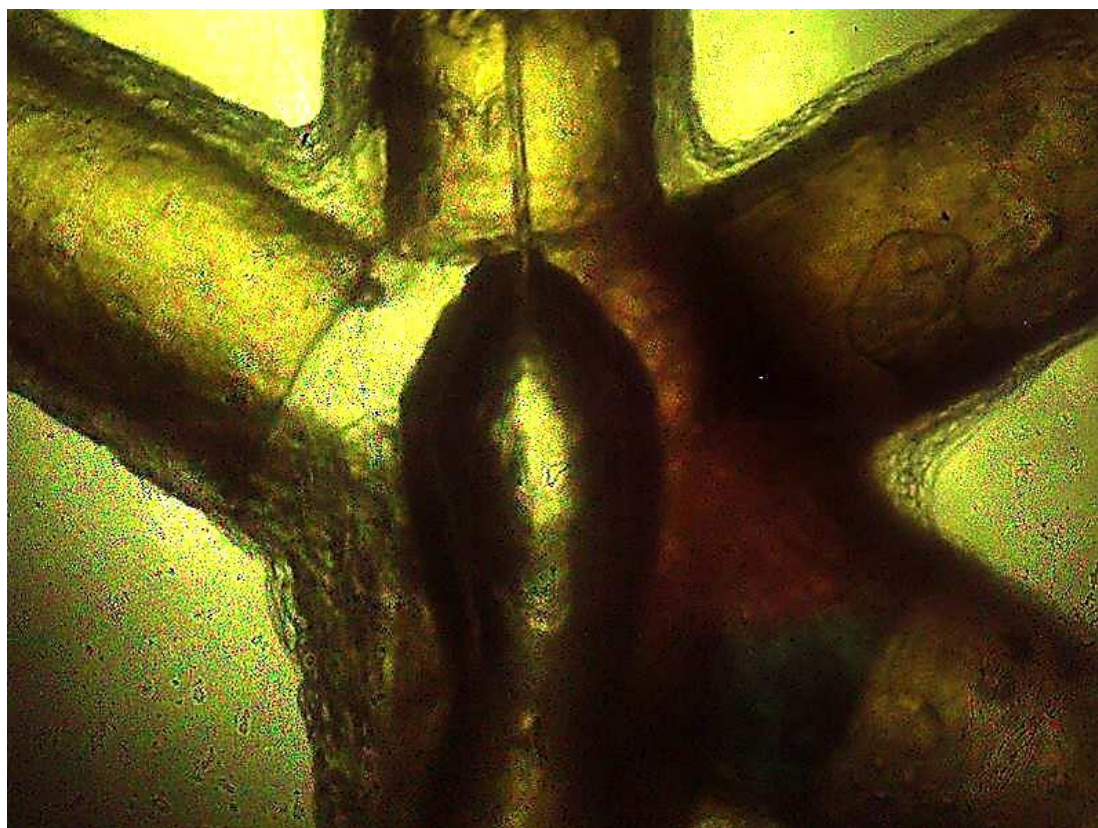
Figure 6.11 Image of periodic flow in the K- junction mixing area captured by high speed camera with solutions (PLGA, PMSQ and PEG) containing three different dyes which are recognised as yellow (left), red (top right) and blue/green (bottom right) respectively.
