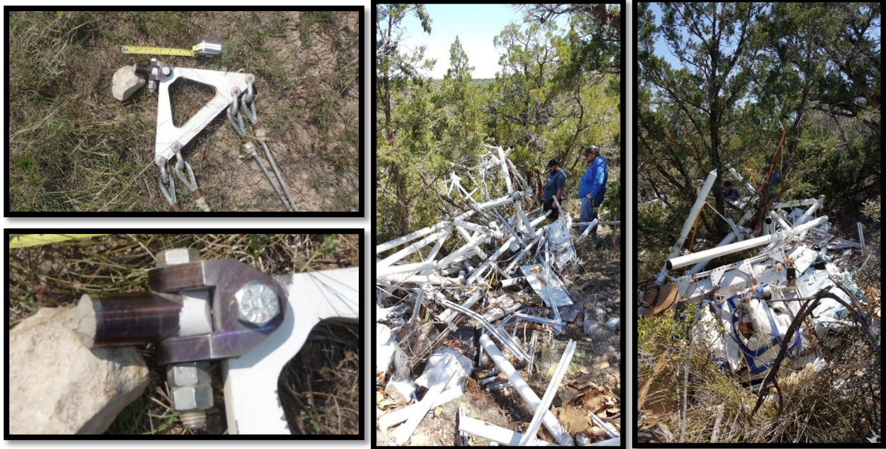
Figure 7: BETTII fell 135,000 feet in ~12 minutes: it did not survive impact. The left two pictures show the truck plate attached to the parachute, along with the rotator pin. The right two pictures show the remnants of the payload.
