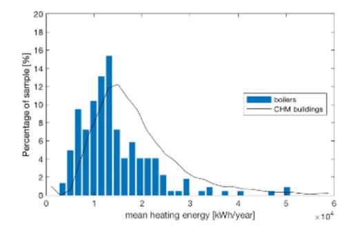
Figure 5: Annual building space heating energy demand derived from boiler data compared to modelled space heating demand of the English housing stock (Field data & CHM<sup>41</sup>)
