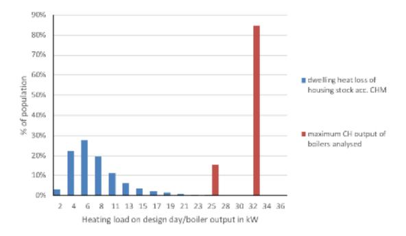
the built stock, given this context it is likely that a significant number of boilers in the analysis dataset are oversized with respect to space heating.
