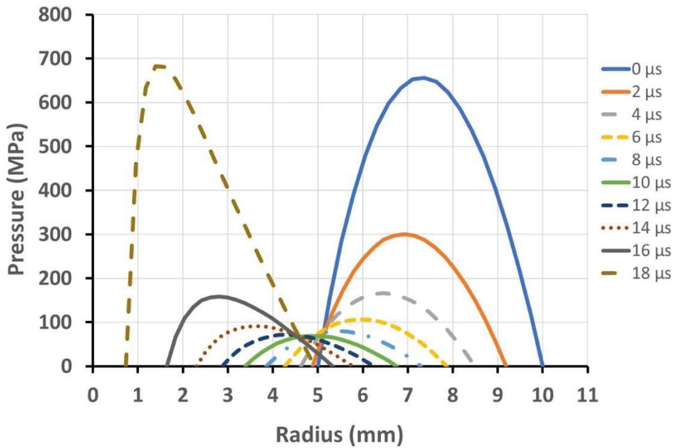
FIGURE 2. Evolution of pressure distribution across jet with time for  $\dot{a}(0) = 0$ .
