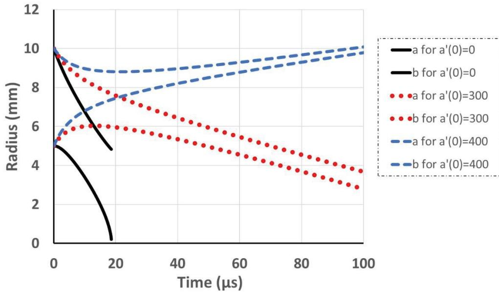
FIGURE 1. Evolution of inner and outer radii with time for different values of  $\dot{a}(0)$ .
