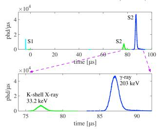
FIG. 4. The time trace, using 10 ns samples, in LUX summed across all 122 PMTs for a <sup>127</sup>Xe decay event with K-shell electron capture in LUX data (top). The event appears as a clear double scatter. An S1 signal is followed by two well separated S2s. The first (green) S2 is due to K-shell x-ray ER, and the second (blue) S2 is due to the 203 keV gamma-ray ER in the LXe volume. The two S1s from both ERs overlap and appear as one S1 (cyan). The (bottom) plot is a closeup of the two S2s.
