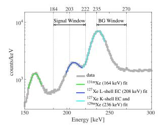
FIG. 9. The reconstructed energy spectrum of single-scatter events in the energy range of interest. The "Signal Window" indicates the energy range where N-shell x-ray signals (Fig. 8 solid blue) are exploited, while "BG Window" indicates the energy range where the N-shell x-ray calibration background model (Fig. 8 solid red) is defined.
