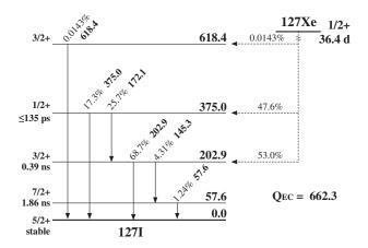
FIG. 1. Decay scheme of <sup>127</sup>Xe [25] with units of keV. The <sup>127</sup>Xe decays via electron capture to <sup>127</sup>I. The percentage above the transition arrow is the gamma-ray intensity as a fraction of parent (<sup>127</sup>Xe) decay.
