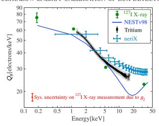
FIG. 10. The  $Q_y$  mean values (green points) measured from  $^{127}$ Xe EC events (this work) at 180 V/cm. The red bar indicates the systematic uncertainty on the  $^{127}$ Xe measurement due to  $g_2$ . Also shown are the  $Q_y$  measured from the LUX tritium calibration [21] at 180 V/cm, of the NEST v0.98 model [11] at 180 V/cm, and measured by the neriX experiment [35] at 190 V/cm. The light gray band on the tritium measurement indicates the systematic uncertainty due to  $g_2$ .
