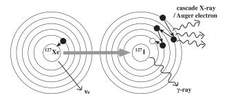
FIG. 2. A schematic illustrating atomic electron capture (a K-shell electron in this case), for a <sup>127</sup>Xe nucleus, which is converted into <sup>127</sup>I in an excited state. The excited <sup>127</sup>I nucleus can subsequently deexcite via emission of one or more gamma rays (or IC electrons). The atomic structure deexcites through x-ray (or Auger electron) cascade emissions.
