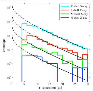
FIG. 6. Histograms of vertical separation (1  $\mu$ s is equivalent to 1.51 mm) between two vertices of EC events with the 203 keV gamma-ray emission for K-(cyan), L-(red), M-(green), and N-(blue) shell x rays. The distributions are fitted with the model described by Eq. (1). The solid black curves are the fits to data. The dashed black curves are the extrapolations from those fits.
