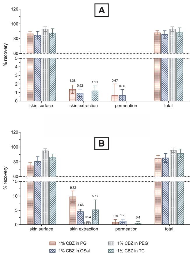
Fig. 5. Percentage of CBZ recovered from applied dose after mass balance in (A) abdominal human skin finite dose application of 1% (w/v) CBZ in PG, OSal, PEG and TC (B) porcine ear skin finite dose application of 1% (w/v) CBZ in PG, OSal, PEG and TC.  $4 \leq n \leq 8$ , mean  $\pm$  SD.
