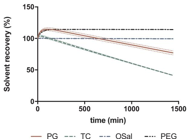
**Fig. 3.** Percentage of weight loss from 1% CBZ solutions in PG, TC, OSal and PEG as prepared for infinite and finite permeation studies.  $n = 3$ , mean  $\pm$  SD.
