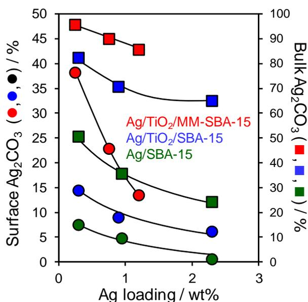
**Figure 4.** Surface (XPS) and bulk (XANES) silver speciation as  $\text{Ag}_2\text{CO}_3$  of Ag/SBA-15, Ag/TiO<sub>2</sub>/SBA-15, and Ag/TiO<sub>2</sub>/MM-SBA-15 as a function of Ag loading.
