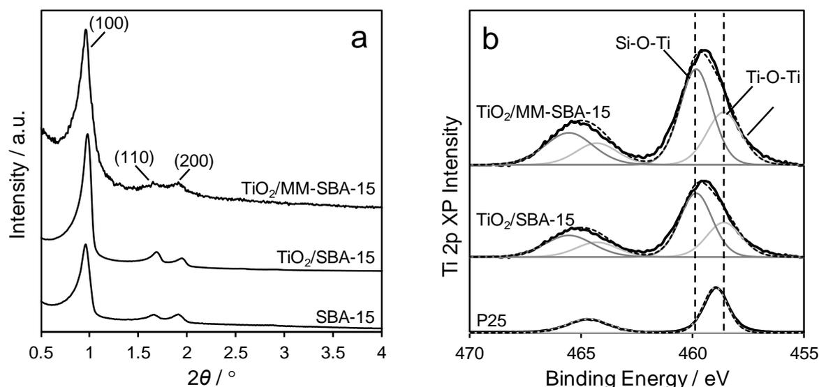
**Figure 3.** (a) Low angle X-ray diffraction (XRD), and (b) fitted Ti  $2p$  XP spectra of  $\text{TiO}_2/\text{SBA-15}$  and  $\text{TiO}_2/\text{MM-SBA-15}$ , alongside pure silica (SBA-15) and titania (P25) references.
