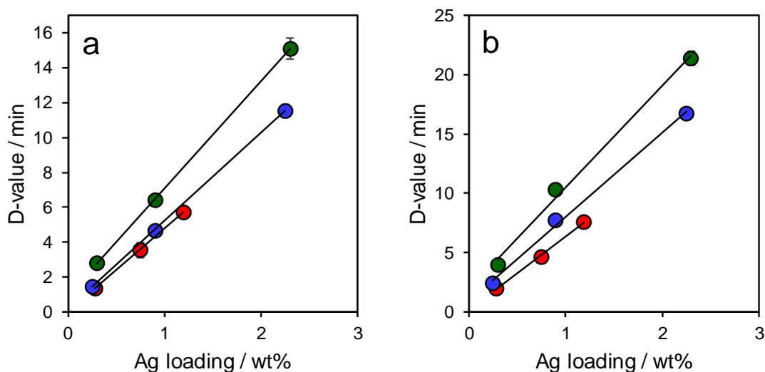
**Figure 7.** Decimal reduction times for Ag/TiO<sub>2</sub>/MM-SBA-15, Ag/TiO<sub>2</sub>/SBA-15 and Ag/SBA-15 against (a) *Staphylococcus aureus*, and (b) *Pseudomonas aeruginosa*.
