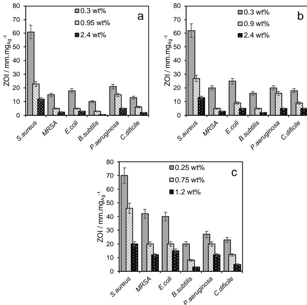
**Figure 6.** Zone of inhibition plots, normalized to mass of Ag, against a range of Gram-positive and Gram-negative bacteria for (a) Ag/SBA-15, (b) Ag/TiO<sub>2</sub>/SBA-15 and (c) Ag/TiO<sub>2</sub>/MM-SBA-15.
