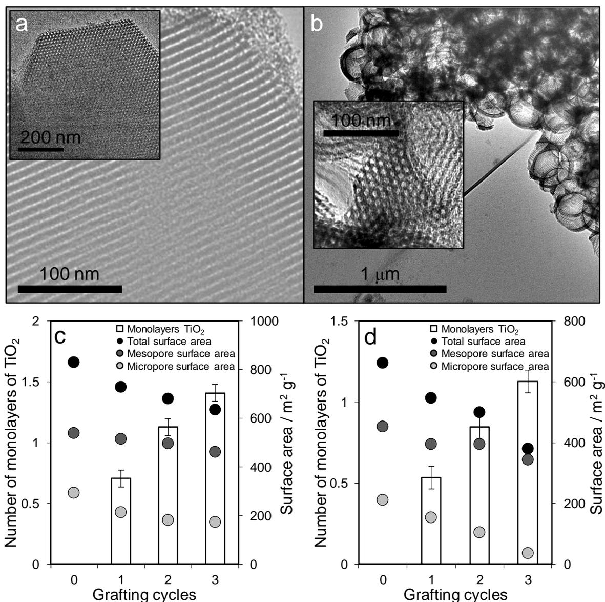
**Figure 2.** Bright-field transmission electron microscopy (TEM) images of (a)  $TiO_2$ /SBA-15 (3<sup>rd</sup> cycle grafting), and (b)  $TiO_2$ /MM-SBA-15 (3<sup>rd</sup> cycle grafting) highlighting ordered hexagonally close-packed mesopores and uniform macropores, and the evolution of textural properties and calculated  $TiO_2$  monolayer thickness as a function of grafting cycle for (c)  $TiO_2$ /SBA-15 and (d)  $TiO_2$ /MM-SBA-15.
