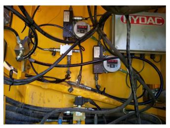
Fig. 3. Particle sensors and external data logger installations.
