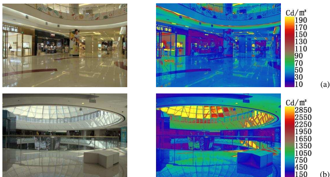
Fig. 1. The HDR images and falsecolor images of two atriums in the shopping centres. (a) An atrium without daylight; (b) An atrium with daylight.
