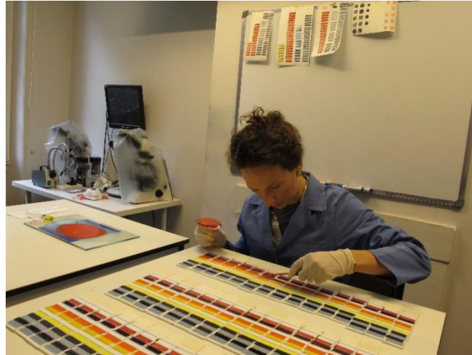
Figure 1. Preparation of oil paint samples
