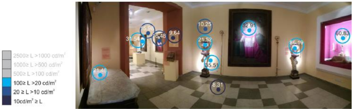
Fig. 6 - Points and values of luminance measured in scene N°5 in the 2st museum
