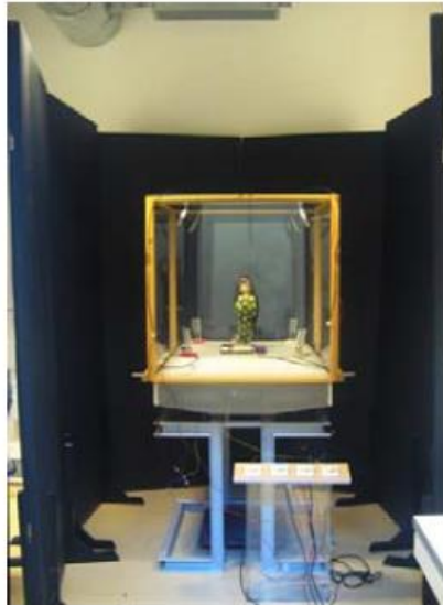
Figure 1 - The pedestal “free-standing” showcase and the experimental set-up.
