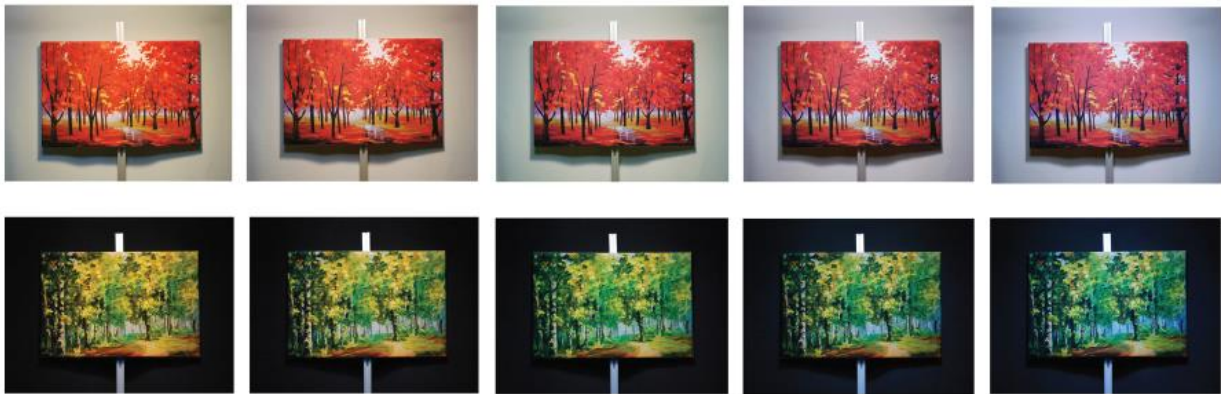
Fig. 5 - Pictures of the red painting on the white background and the green painting under the black background under the various configurations (from warm to cool CCT).
