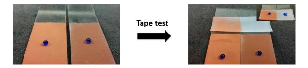
Fig. 5.9 Tape adhesive test of the uncoated and coated S.H-Cu samples (from left to right).
