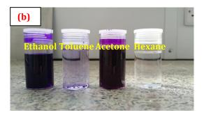
**Fig. 2.2** (a) Crystal violet-incorporated polymer sections prepared by immersion in crystal violet/ organic solvent swelling solutions for 24 h (immediately post-removal from swelling solution. Organic solvents used are as follows: 1. water, 2. ethanol, 3. methanol, 4. acetone, 5. toluene, 6. hexane, 7. chloroform, 8. THF. (b) Polymer sections immersed in different crystal violet/ organic solvent swelling solutions (100 % solvent).
