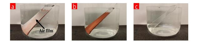
**Figure 5.5** (a) The SH glass surfaces is capable of trapping air in aqueous environment, leading to an underwater air-film. (b) and (c) In comparison, the air-film cannot be stabilized by the SLIP and plain glass samples.
