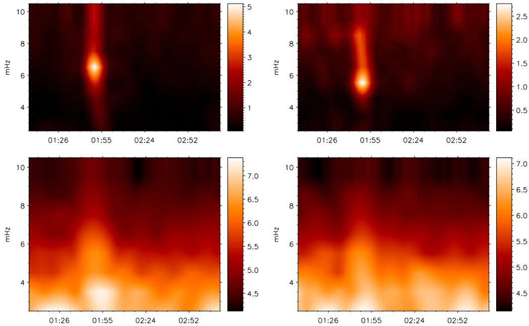
**Figure 4.** Frequency response for Source 1 (left) and Source 2 (right). Egression power rms as function of time (along  $x$ -axis) and frequency (along  $y$ -axis) are plotted in units of quiet-Sun egression power (top row) and as  $\log_{10}$  of acoustic energy flux [ $\text{erg cm}^{-2} \text{s}^{-1}$ ] (bottom row) for corresponding frequency band.
