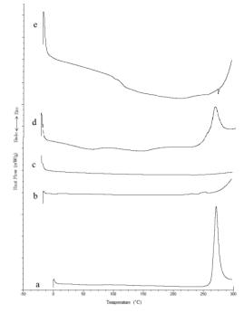
Figure 4: DSC Thermograms of – a) Rif; b) chitosan; c) OC;d) OC-Rif physical mixture; e) OC-Rif NPs
