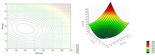
Figure 1; (a) Contour plot showing the effect of independent factors on mean particle size (MPS); (b) Response surface plot showing the effect of independent factors on MPS
