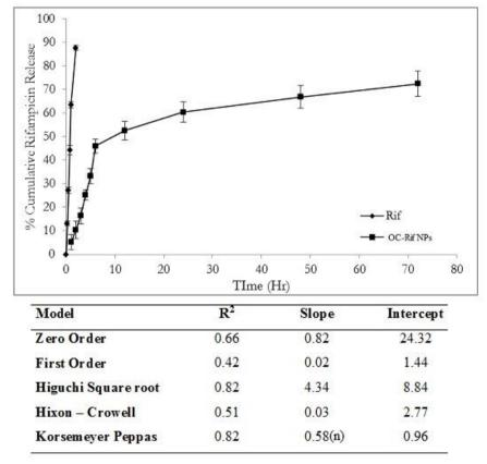
**Figure 6:** Percent cumulative release of Rif from OC-Rif nanoparticles  $(n=3, mean \pm SD)$
