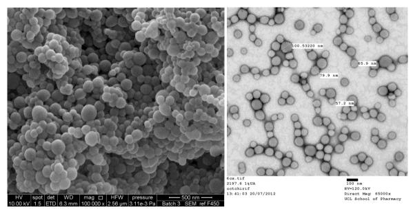
Figure 3; a) Scanning electron micrograph of OC-Rif NPs ; b) Transmission electron micrograph of OC-Rif NPs
