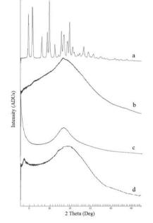
**Figure 5:** X-Ray diffratograms of – a) Rif ; b) Chitosan c) OC; d) OC-Rif NPs
