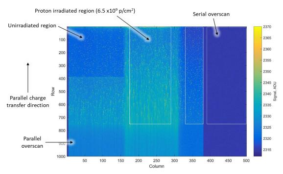
Figure 4. Binned readout from one node of a PLATO CCD270, which has had regions irradiated with protons. This image was recorded with exposure to a 55Fe source, with the detector at 207 K.
