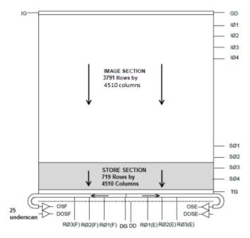
Figure 3. Schematic layout of the SMILE SXI CCD370.
