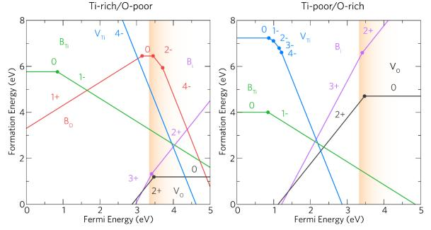
Figure 8. The transition level diagrams for  $TiO_2$ :B under both Ti-rich/O-poor (left) and Ti-poor/O-rich (right) growth regimes. The Fermi energy goes from the VBM (0 eV) to 1.7 eV above the CBM (which is at 3.35 eV). The conduction band region is shown by the graded.
