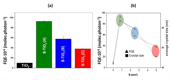
Figure 6. (a) Formal quantum efficiencies (FQE) obtained during photodegradation of stearic acid under UVA irradiation of undoped and boron-doped  $TiO_2$  films (**Table 1**); (b) comparison between photocatalytic activities and crystallite sizes as determined from XRD analysis. Crystal size data presented in table 1.
