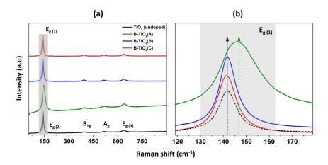
Figure 3. (a) Raman spectra of the  $TiO_2$ :B samples, compared to the undoped anatase film and (b) Raman shift of the Eg band zoomed. Black dotted arrow (left) indicates the position of the undoped  $TiO_2$  and dotted green arrow (right) the position of the Eg(1) band for  $TiO_2$ : (A).
