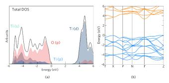
Figure 7. The calculated density of states (DoS) (a) and band structure (b) of undoped anatase  $TiO_2$ . In each diagram the valence band maximum (VBM) is set to 0 eV. In (b) the valence bands are depicted as blue lines and the conduction bands as orange lines.
