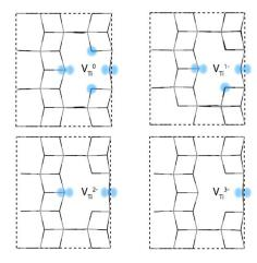
Figure 9. The partial charge densities of the charge states of  $V_{Ti}$  as viewed along the {010} direction showing the localisation of holes (blue isosurfaces) in each example. The isosurfaces are plotted from 0 - 0.015 eV Å-3.
