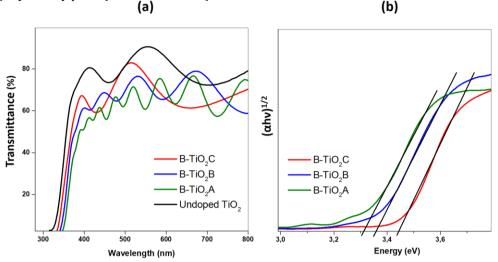
Figure 5. (a) UV-visible spectra (transmittance) of the doped and undoped  $TiO_2$  films, (b) graphical calculation (Tauc plot) of the optical band gap for all the boron-doped  $TiO_2$  samples.
