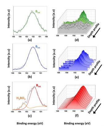
Figure 1. B 1s XPS surface and in depth profile spectra of  $TiO_2$ :B samples: (a)  $TiO_2$ :B (A); (b)  $TiO_2$ :B (B) and (c)  $TiO_2$ :B (C); (d, e and f) depth profiling spectrum of  $TiO_2$ :B (A),  $TiO_2$ :B (B),  $TiO_2$ :B (C) thin films, respectively. Dashed black lines in figures a, b and c represent the raw data (CPS) in XPS.
