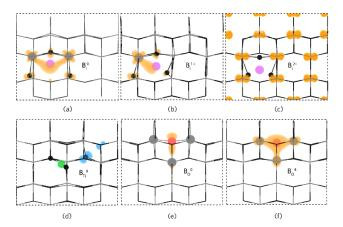
Figure 10. The partial charge densities of  $B_i^0$  (a),  $B_i^{1+}$  (b),  $B_i^{2+}$  (c),  $B_{Ti}^0$  (d),  $B_0^0$  (e) and  $B_0^{4-}$  (f) defect charge states as viewed along the {100} direction displaying the localisation of holes and electrons (blue and orange isosurfaces respectively). The isosurfaces are plotted from 0-0.015 eV Å<sup>-3</sup>.
