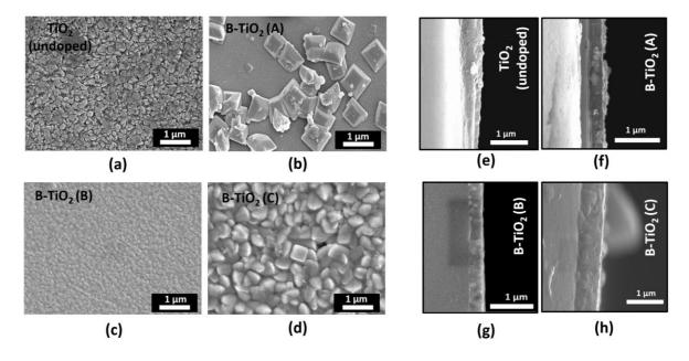
Figure 4. SEM images (top view) of: (a) Undoped TiO<sub>2</sub>, (b) TiO<sub>2</sub>:B (A), (c) TiO<sub>2</sub>:B (B) and (d) TiO<sub>2</sub>:B (C); Cross-section SEM images (e, f, g and h) of the undoped and boron-doped thin films, respectively.
