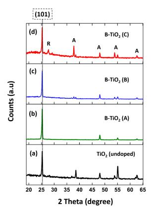
Figure 2. XRD patterns of undoped and B-doped  $TiO_2$  thin films (A = anatase and R = rutile); (a) undoped  $TiO_2$ ; (b) sample  $TiO_2$ :B (A); (c) sample  $TiO_2$ :B (B); (d) sample  $TiO_2$ :B (C). Dotted line represents the crystalline plane (101) of anatase.
