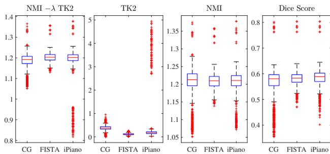
**Fig. 2.** 3D-Comparison of FISTA and iPiano against the conjugate gradient (CG) solver based on overall 1180 registrations. The Dice scores represent the mean of all propagated labels for each registration. All FBS results, apart from NMI, are statistically significantly better ( $p < 10^{-6}$ ) than the CG ones based on the Wilcoxon signed rank test.
