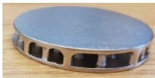
Figure 1. An AM produced aluminium sample of 4 cm diameter with a simple arches support structure. 4
