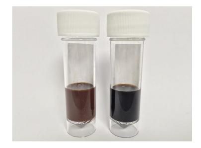
**Figure 4.1.** Raw vinasse before (left) and after (right) suspended solids separation. Suspended solids removal by centrifugation as described in Section 2.3.2.
