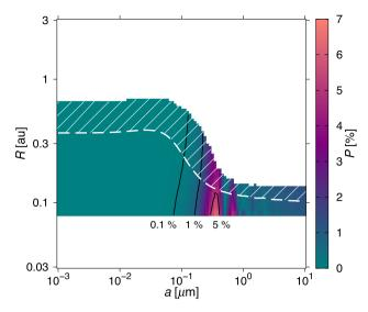
**Figure 5.** Polarization degree P of the total radiation for the system HD 56537. The dashed white line indicates the sublimation radius and the region of suitable parameter settings is highlighted as dashed area (see Fig. 4). The black contour lines show the 0.1 per cent, 1 per cent and 5 per cent levels. The dust material is graphite and the inclination is  $90^{\circ}$ .
