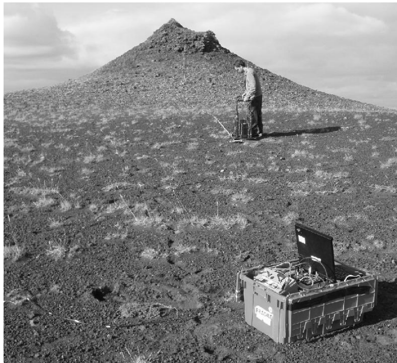
Figure 4.3. Configuration of the GPR setup during surveying. The box containing the car battery, processing station, and laptop is in the foreground. This is connected via optic fibre cables to the transmitter and receiver antennas being moved in constant increments along the survey line in the background.
