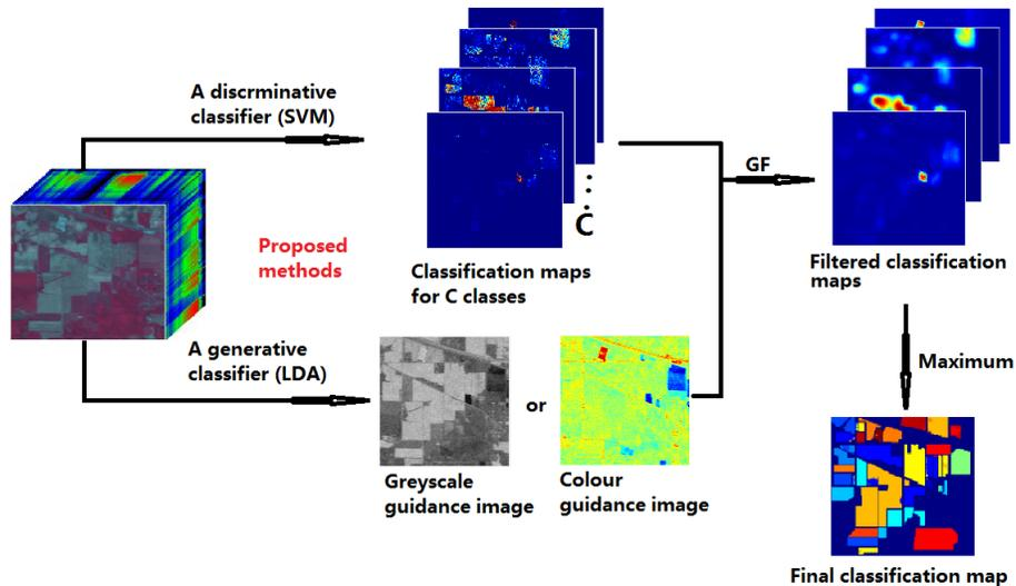
Figure 1: The proposed DGF methods for HSI classification.
