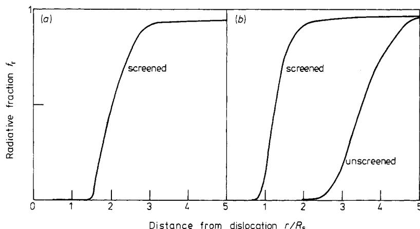
**Figure 4.** Radiative fraction of luminescent centres as a function of distance from dislocation
