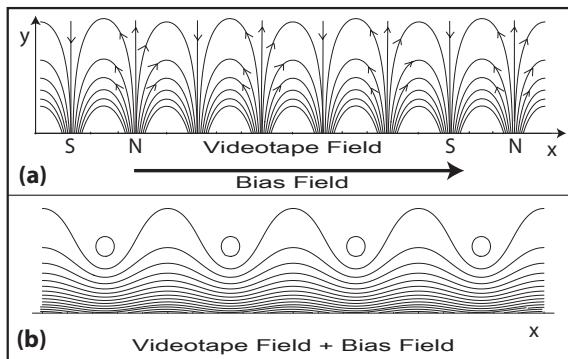
**Figure 1.** (a) Videotape magnetic field lines and uniform bias field. (b) Contours of constant field strength once the bias field is added. Weak-field-seeking atoms can be trapped in the circular minima.
