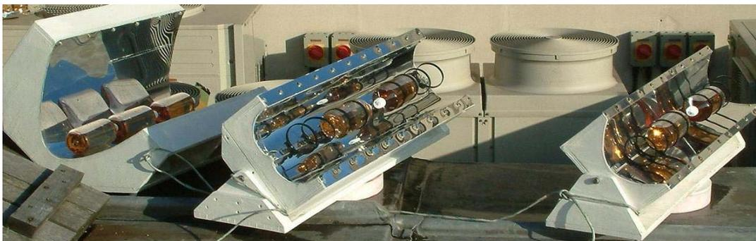
**Figure 4.4** Solar irradiation experimental set-up on the roof of Chadwick Building, UCL, London. From left to right: bigger parabolic collector (BPC), compound parabolic collector (CPC) and parabolic collector (PC).
