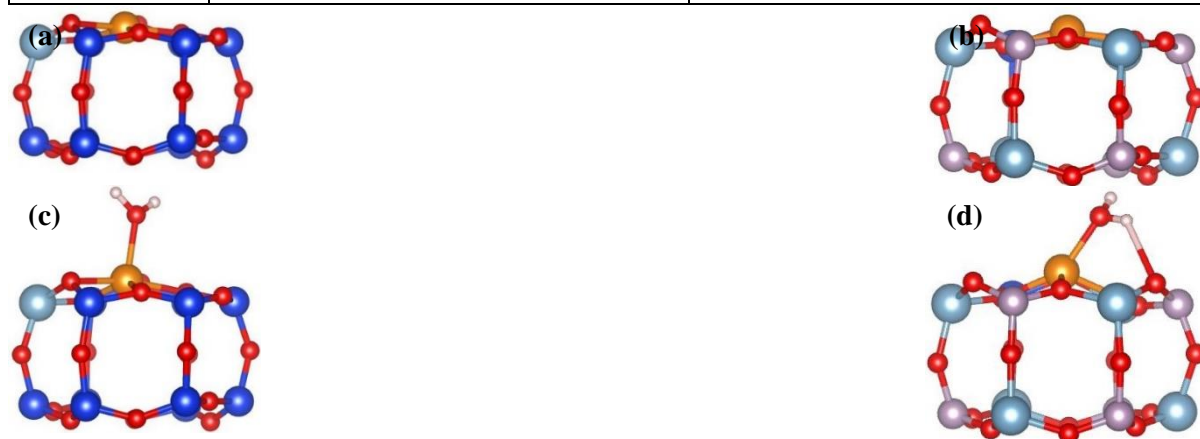
Figs. 55(a – d): (a – b) (110) view of the Cu inside the 6MR of site SI in the single configuration before H 2 O coordination, and (c – d) after coordination.
