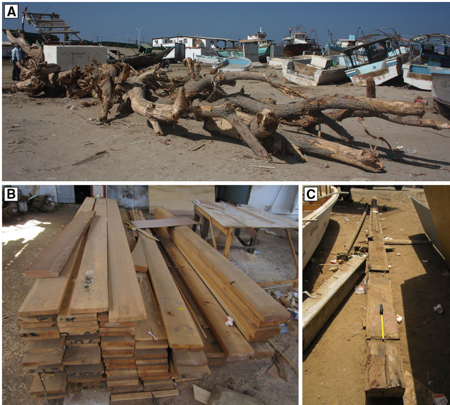
Fig. 11 Timbers at the yard of Ibrahim Bilghaith, al-Hafa, Jizan: a Unworked neem crooks (Image: J. P. Cooper); b Imported pre-cut planks of Swaydi ('Swedish') timber, identified from samples as pine ( Pinus spp) (Image: L. Semaan); c Disarticulated keel made of teak at the Bilghaith yard, al-Hafa, Jizan (Image: L. Semaan)
