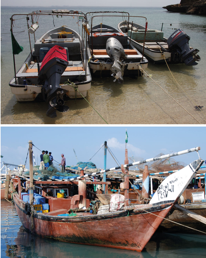
Fig. 8 Above Imported fibreglass falūkas with outboard motors at Sadayn, Greater Farasan (Image: J. P. Cooper); Below fibreglass-coated vessels modelled on the Omani and Arabian-Persian Gulf shū ṭ are the mainstay of the contemporary Jizan fishing fleet (Image: Peter Harrigan)
