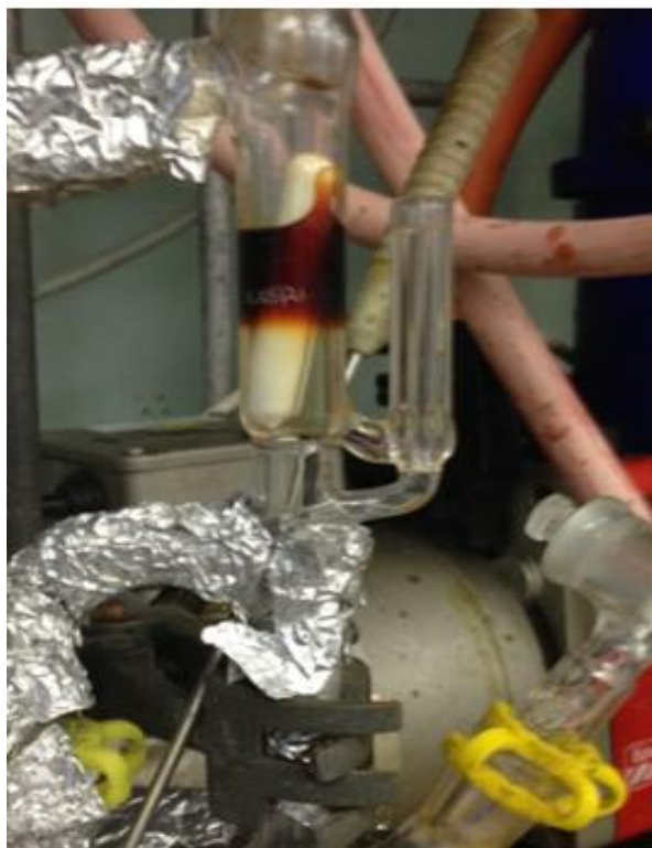
Figure 57: Gravex 926 with \text{TiCl}_4 during first cycle. The red distillate is seen to gather on top off the clean \text{TiCl}_4 that starts off in the Soxhlet, before falling though when it fills.
