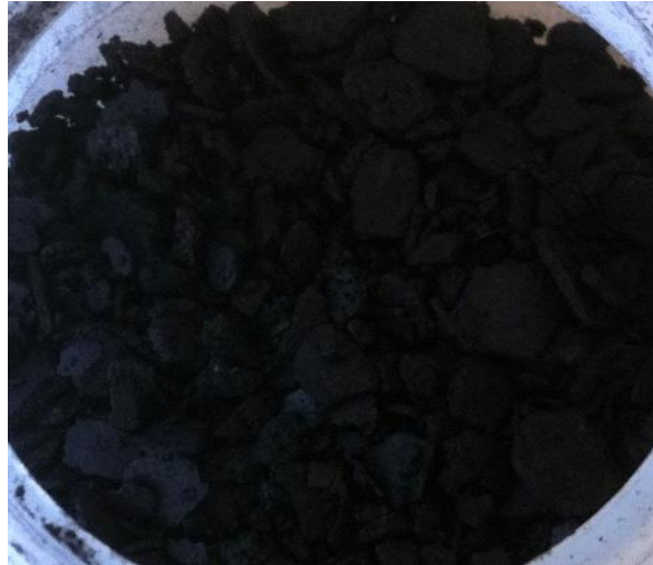
Figure 7: Collected black residue in the furnace, following cleaning.
