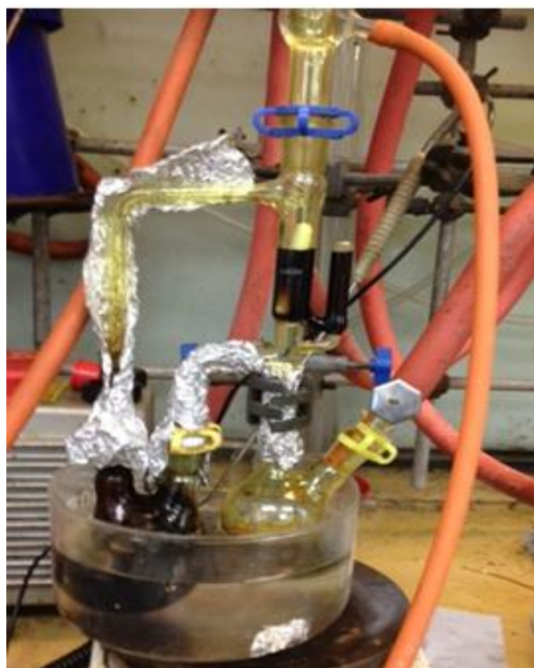
Figure 58: 25ml \text{TiCl}_4 and 1ml \text{VOCl}_3 with Flavex 977(s). Flow system is stained; solid in Soxhlet suggests that whatever carries over continues reacting.
