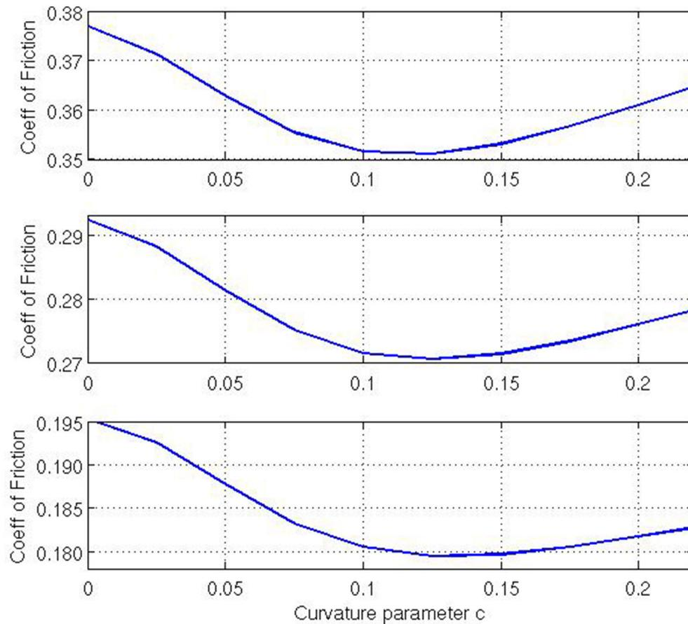
**FIGURE 6 | Coefficient of friction relative to lateral curvature parameter  $c$  where the geometry has non-negative Gaussian curvature. Top:  $\tau_{max}/\tau_0 = 2.00$ , Middle:  $\tau_{max}/\tau_0 = 1.75$ , Bottom:  $\tau_{max}/\tau_0 = 1.50$ .**
