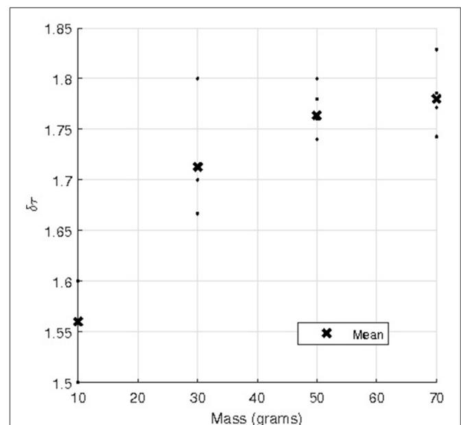
**FIGURE 3 | Tension ratio against applied mass from the raw experimental data in Table 1 obtained from Karavokiros (2007).**
