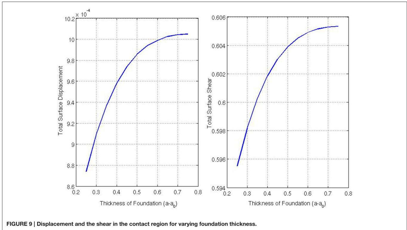
FIGURE 9 | Displacement and the shear in the contact region for varying foundation thickness.
