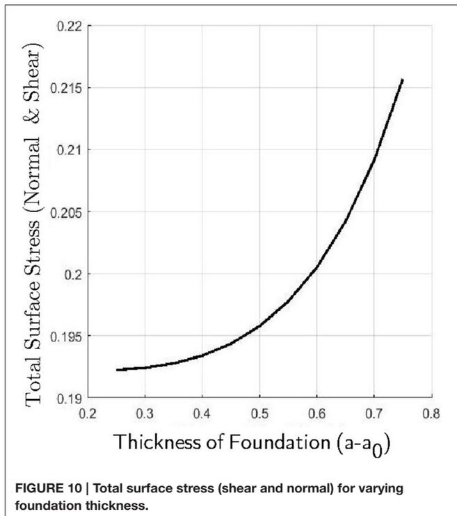
FIGURE 10 | Total surface stress (shear and normal) for varying foundation thickness.
