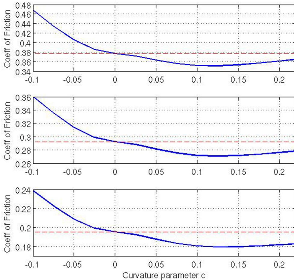
**FIGURE 7 | Coefficient of friction relative to  $c$  including geometries with positive and negative Gaussian curvature. Top:  $\tau_{\max}/\tau_0 = 2.00$ , Middle:  $\tau_{\max}/\tau_0 = 1.75$ , Bottom:  $\tau_{\max}/\tau_0 = 1.50$ .**
