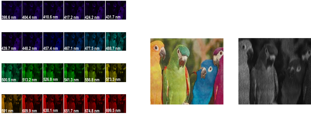
Fig. 9. Left: hyperspectral image (reference). Middle: RGB image. Right: CASSI measurement.
