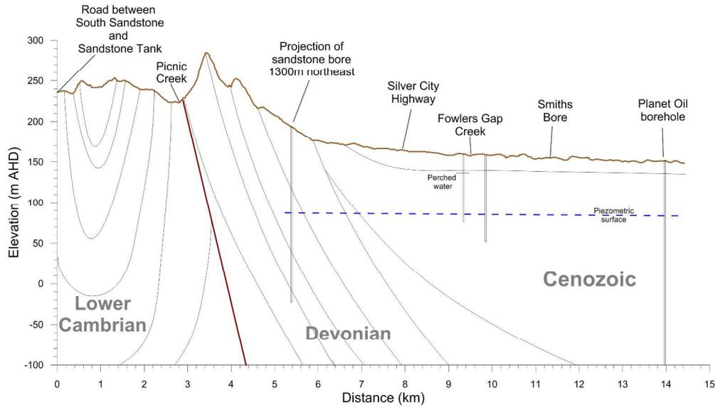
Figure 3: Sketch section showing general geological units and basic groundwater level data at FGAZRS. Line of section is shown in Figure 1b.
