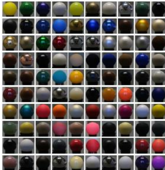
Figure 2.13: Material samples used to measure BRDFs for the MERL database. Image: http://www.merl.com/brdf/
