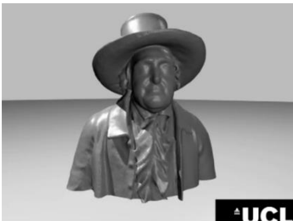
Figure 2.5: A 3D model of Jeremy Bentham's auto icon created by UCL's 3DImpact group using a Kinect scanner and ReconstructMe software. Further work was carried out on the model in Meshlab. See http://www.youtube.com/watch?v=Gy7muFzA1e0 , and more information found at http://uclgeomatrics.com/2012/11/09/jeremy-bentham-in-3d/
