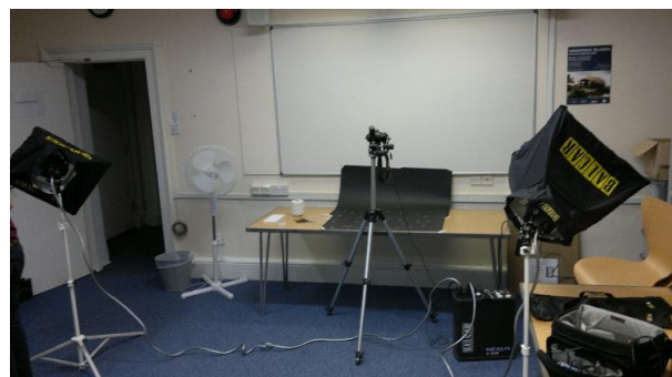
Figure 6.10: Camera setup, wide view, including the two lights with soft boxes
