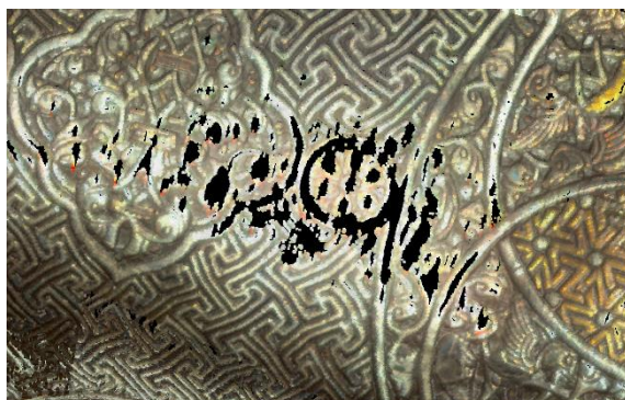
Figure 6.5: Holes in the laser scan caused by excessive reflection
