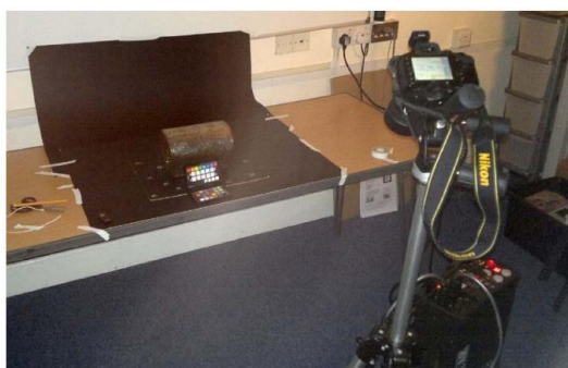
Figure 6.9: Setup for capturing photogrammetry images – note the colour chart in front of the bag
