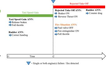
Fig. 7. (Rejected Take Off experiment) The behaviour of the IAS when engine(s) failure or fire is detected and a Rejected Take Off (RTO) is performed. The Fire Situation ANN is used only when fire is detected.
