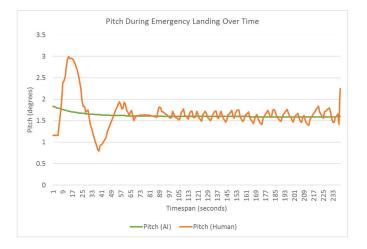
Fig. 8. (Emergency landing experiment) A comparison between the human pilot and the Intelligent Autopilot System's pitch during emergency landing. In this case the human pilot struggled to generate perfect training data so our training approach was designed to prevent overfitting, instead creating a general model (good fit) which provided the desired performance.
