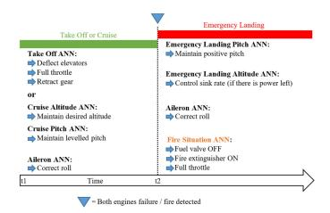
Fig. 10. (Emergency landing experiment) The behaviour of the IAS when both engines failure or fire is detected during either take off or cruise, and an emergency landing is performed. The Fire Situation ANN is used only when fire is detected.
