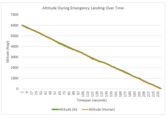
Fig. 9. (Emergency landing experiment) A comparison between the human pilot and the Intelligent Autopilot System's altitude during emergency landing. The results show a significantly close sink rate of about 1500 ftagl per minute.
