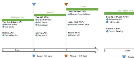
Fig. 6. The behaviour of the IAS when controlling the transition of flight modes under normal conditions. Different ANNs are used in each flight mode.
