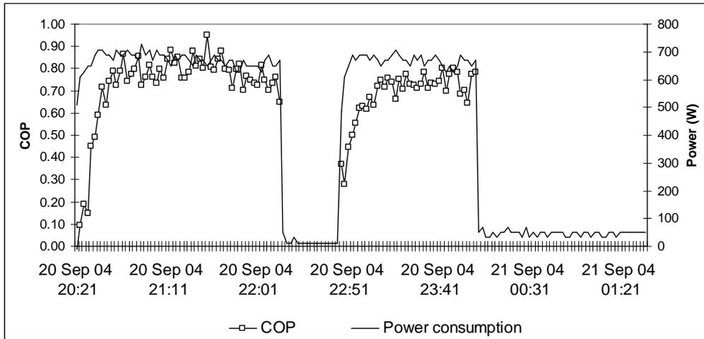
**Figure 3:** Monitored EER and Power Drawn for the Portable Unit
