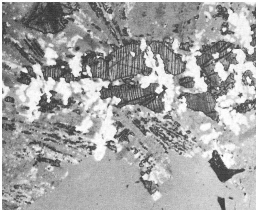
Figure 52 – Photomicrograph of a typical blast furnace slag in thin section (Magnification x300) Source: Lee (1974))
