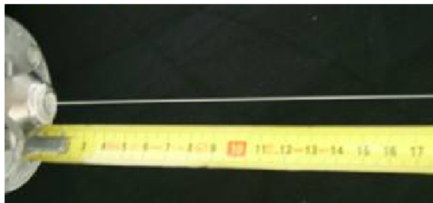
Figure 5.2.4: Picture showing a stable fluid jet of a nozzle applying hydraulic flip.
