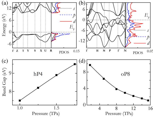
FIG. 4 (color online). Electronic band structure and projected density of states of *oP8*-Na at 1.75 TPa (PDOS, in units of  $\text{eV}^{-1}$  per atom) (a) and *cI24*-Na at 16 TPa (b). The horizontal dotted lines indicate the Fermi level. [(c) and (d)] Variation of band gaps with pressure for *hP4* and *oP8*-Na, respectively, using the HSE06 functional.
