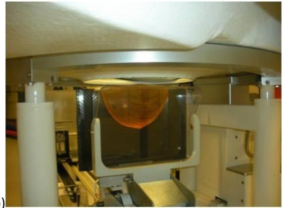
**Figure 1 Elettra SYRMEP beam-line experimental setup.** Figure adopted from (<http://www.elettra.trieste.it>), modified and mammography facility at SYRMEP beamline: patient support (b) and positioning of the biopsy phantom (c)
