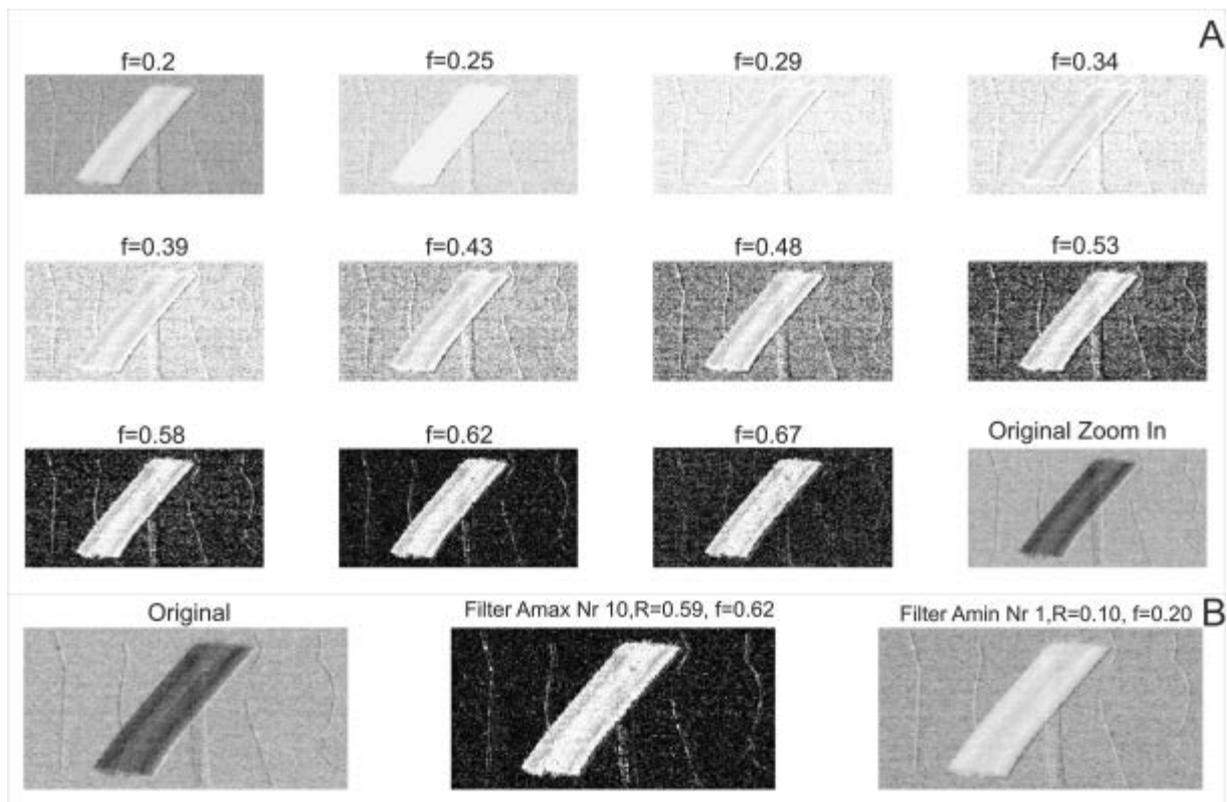
FIG. 2 A. FREQUENCY DECOMPOSITION PROCESS. AN INTEGRATION OF THE ORIENTATION DECOMPOSITION PROCESS FOR THE RANGE  $= 0 - 135^\circ$  LEADS TO SERIES OF IMAGES FOR THE RANGE OF SCANNED FREQUENCIES. IMAGES ARE LABELLED WITH THE FREQUENCY. AT SOME FREQUENCIES, THE INTENSITY RATIO BETWEEN OBJECTS (WIRES, PLASTICS) AND BACKGROUND APPROACHES 300 %. THE UNPROCESSED IMAGE IS ALSO SHOWN FOR COMPARISON (WITH THE TITLE 'ORIGINAL ZOOM IN').
