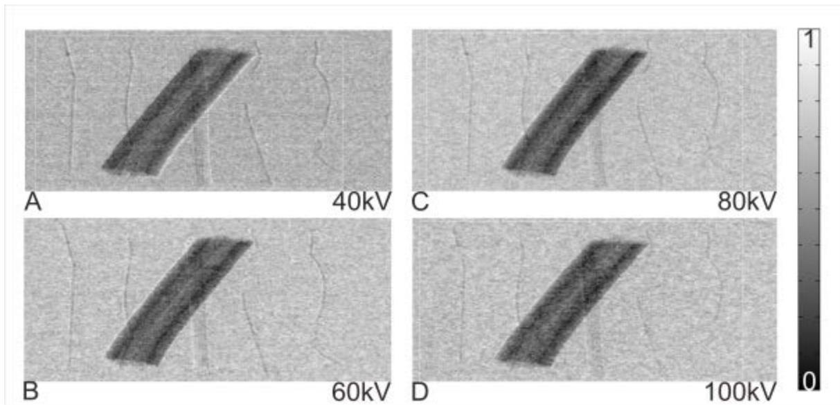
FIG. 1 X-RAY PHASE CONTRAST IMAGES OF THE CUSTOM BUILT PHANTOM SIMULATING A PLASTIC EXPLOSIVE DEVICE PLUS VARIOUS BINDING FIBRES AND THIN METALLIC WIRES (SEE TEXT). IMAGES A, B, C AND D WERE ACQUIRED AT INCREASING X-RAY TUBE VOLTAGES, AS LABELLED.
