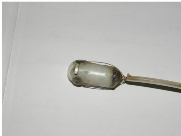
Fig. 4.20 Bidirectional video capsule endoscope
