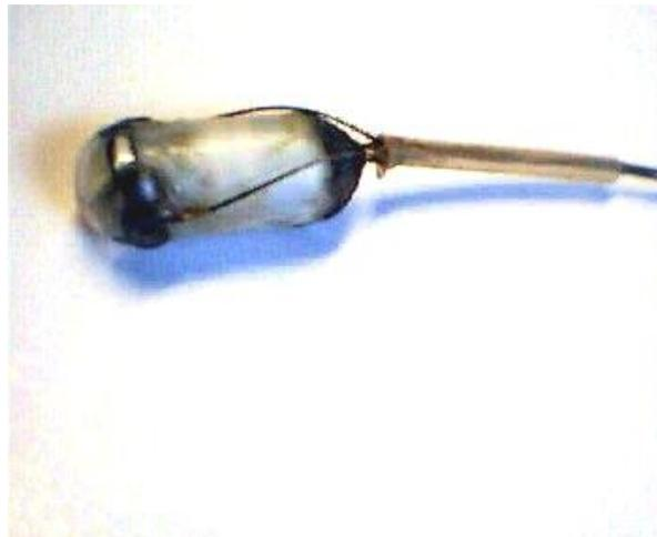
Fig. 4.18 Double Ended video capsule endoscope
