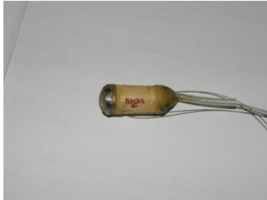
Fig. 4.19 Bidirectional video capsule endoscope
