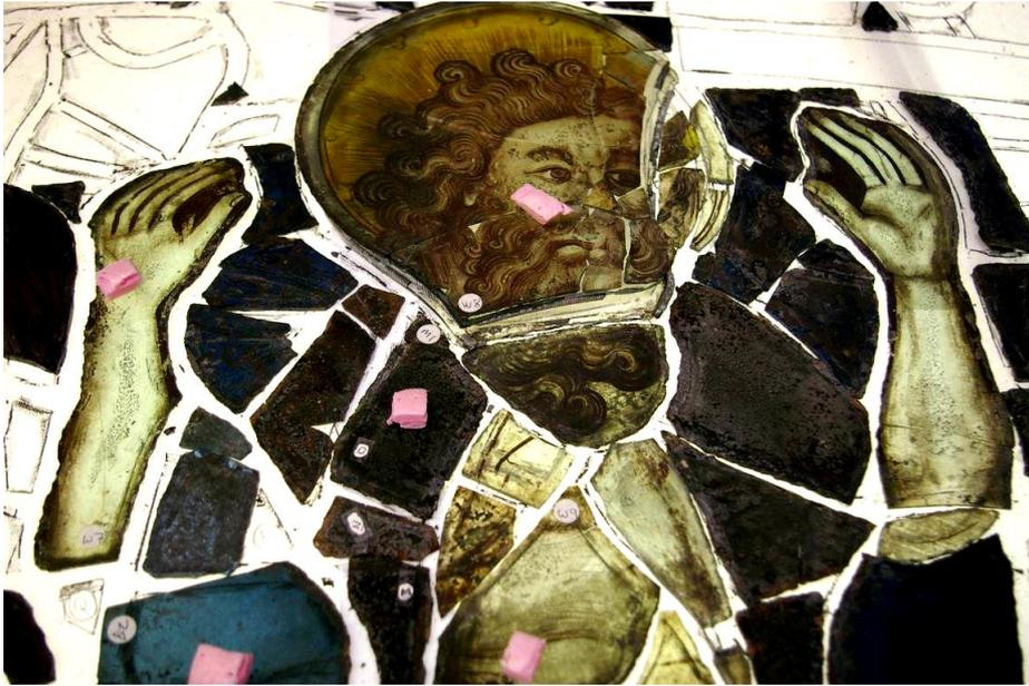
Fig. 2. Panel 2e during the sampling process. Small foam blocks are used to indicate fragments to be sampled, and sampling positions indicated by small labels, following discussion amongst YGT conservation staff and members of the project team.
