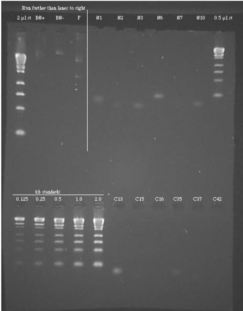
2% agarose electrophoresis of hybrid purified *EcoRI* and *XhoI* cleaved differentially displayed fragments (C13-C42). S (Standard).
