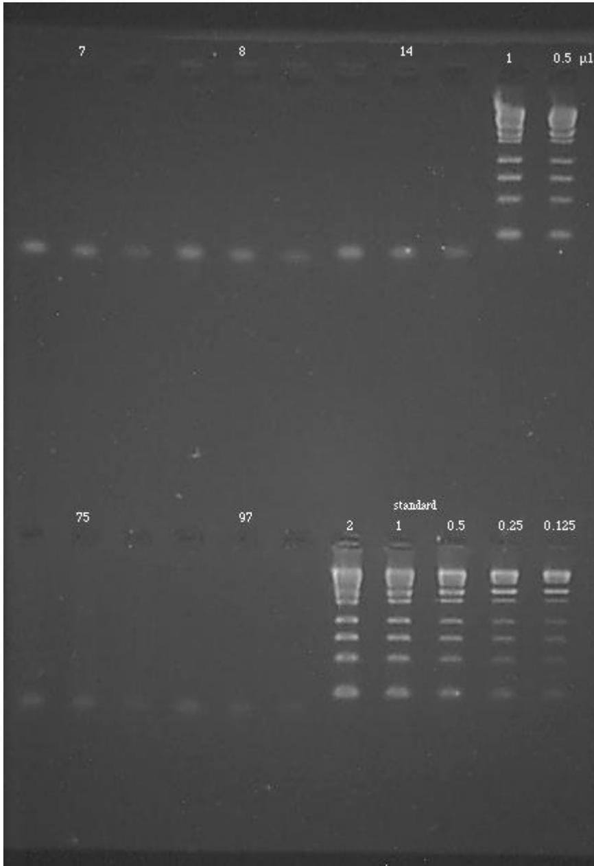
DNA quantitation in Hybaid column purified samples (30µl elutes) each loaded at 2.25, 1.5 and 0.75 µl.
