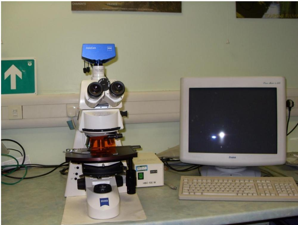
Figure 23: Zeiss Axioskop2 MAT microscope
