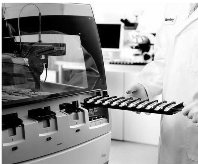
Figure 21: Vision Automated Immunohistochemistry Staining System
