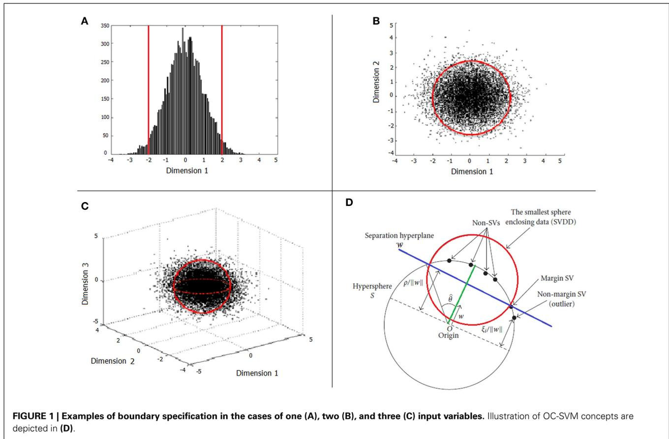
**FIGURE 1 |** Examples of boundary specification in the cases of one (A), two (B), and three (C) input variables. Illustration of OC-SVM concepts are depicted in (D).
